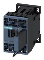
traction contactor, AC-3e/AC-3, 12 A, 5.5 kW / 400 V, 110 V DC, 0.7-1.25\*Us with integrated suppressor diode 3-pole, frame size S00 spring-loaded terminal suitable for PLC outputs not expandable with auxiliary switch
