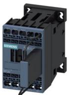
traction contactor, AC-3e/AC-3, 12 A, 5.5 kW / 400 V, 110 V DC, 0.7-1.25\*Us with integrated suppressor diode 3-pole, frame size S00 springloaded terminal suitable for PLC outputs for upright mounting position not expandable with auxiliary switch
