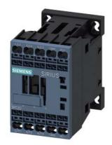
power contactor, AC-3e/AC-3, 12 A, 5.5 kW / 400 V, 3-pole, 24 V DC, 0.7-1.25\* Us, with integrated varistor, auxiliary contacts: 1 NO, spring-loaded terminal, size: S00
