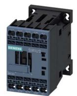
power contactor, AC-3e/AC-3, 12 A, 5.5 kW / 400 V, 3-pole, 24 V DC, 0.7-1.25\* Us, with integrated varistor, auxiliary contacts: 1 NC, spring-loaded terminal, size: S00
