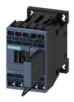
traction contactor, AC-3e/AC-3, 12 A, 5.5 kW / 400 V, 110 V DC  $0.7-1.25^{*}$  Us, with varistor integrated, 3-pole frame size S00, spring-loaded terminal
