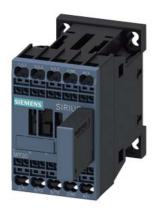
power contactor, AC-3e/AC-3, 12 A, 5.5 kW / 400 V, 1 NC, 24 V DC 0.7-1.25\* Us, with varistor plugged on, 3-pole frame size S00, spring-loaded terminal not expandable with auxiliary switch
