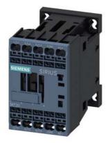
power contactor, AC-3e/AC-3, 12 A,  $5.5~\rm kW$  / 400 V, 1 NC, 24 V DC 0.85-1.85\* Us, with suppressor diode integrated frame size S00, spring-loaded terminal
