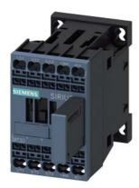
power contactor, AC-3e/AC-3, 12 A, 5.5 kW / 400 V, 1 NO, 24 V DC 0.85-1.85 $^{\circ}$  Us, with varistor plugged on, 3-pole frame size S00, spring-loaded terminal not expandable with auxiliary switch
