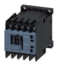
power contactor, AC-3e/AC-3, 12 A, 5.5 kW / 400 V, 1 NC, 24 V AC, 50 / 60 Hz 3-pole, frame size S00 ring cable lug connection
