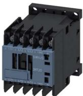
power contactor, AC-3e/AC-3, 12 A, 5.5 kW / 400 V, 1 NO, 110 V AC, 50 Hz, 120 V 60 Hz, 3-pole, frame size S00 ring cable lug connection
