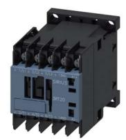
power contactor, AC-3e/AC-3, 12 A, 5.5 kW / 400 V, 3-pole, 24 V DC, 0.7-1.25\* Us, with integrated suppressor diode, auxiliary contacts: 1 NO, ring cable lug connection, size: S00, suitable for PLC outputs, not expandable with auxiliary switch
