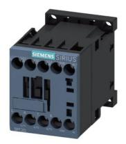
power contactor, AC-3e/AC-3, 7.5 kW/400 V, 1 NC, 100 V AC, 50 Hz, 100  $\dots$  110 V, 60 Hz, 3-pole, frame size S00, screw terminal
