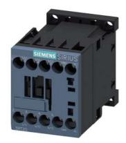
power contactor, AC-3e/AC-3, 7.5 kW/400 V, 1 NO, 110 V AC 50 Hz 120 V 60 Hz, 3-pole, frame size S00 screw terminal
