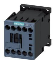
power contactor, AC-3e/AC-3, 16 A, 7.5 kW / 400 V, 1 NC, 220 V AC, 50/60 Hz 3-pole, frame size S00 screw terminal
