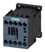
power contactor, AC-3e/AC-3, 16 A, 7.5 kW / 400 V, 1 NO, 400 V AC, 50 Hz 400-440 V, 60 Hz, 3-pole frame size S00, screw terminal
