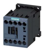
power contactor, AC-3e/AC-3, 16 A, 7.5 kW / 400 V, 1 NO, 277 V AC, 60 Hz 3-pole, frame size S00 screw terminal
