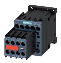
power contactor, AC-3e/AC-3, 16 A, 7.5 kW / 400 V, 2 NO + 2 NC, 24 V DC 3-pole, frame size S00 screw terminal captive auxiliary switch
