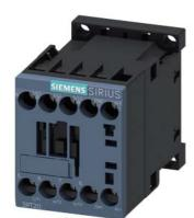
power contactor, AC-3e/AC-3, 16 A, 7.5 kW / 400 V, 1 NC, 24 V DC with diode integrated, 3-pole, screw terminal
