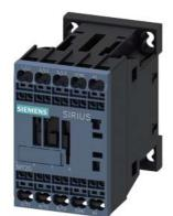
power contactor, AC-3e/AC-3, 16 A, 7.5 kW / 400 V, 1 NC, 42 V AC, 50/60 Hz 3-pole, frame size S00 spring-loaded terminal
