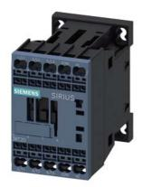
power contactor, AC-3e/AC-3, 16 A, 7.5 kW / 400 V, 1 NC, 48 V AC, 50/60 Hz 3-pole, frame size S00 spring-loaded terminal
