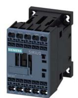
power contactor, AC-3e/AC-3, 7.5 kW/400 V, 1 NO, 110 V AC 50 Hz, 120 V 60 Hz, 3-pole, frame size S00 spring-loaded terminal
