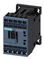
power contactor, AC-3e/AC-3, 16 A, 7.5 kW / 400 V, 1 NC, 220 V AC, 50/60 Hz 3-pole, frame size S00 spring-loaded terminal
