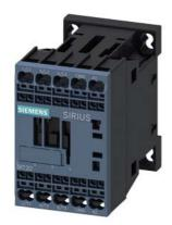
power contactor, AC-3e/AC-3, 16 A, 7.5 kW / 400 V, 1 NO, 220 V AC, 50 Hz, 240 V 60 Hz, 3-pole, frame size S00 spring-loaded terminal
