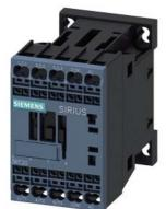
power contactor, AC-3e/AC-3, 16 A, 7.5 kW / 400 V, 1 NC, 220 V AC, 50 Hz, 240 V 60 Hz, 3-pole, frame size S00 spring-loaded terminal
