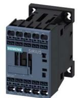
power contactor, AC-3e/AC-3, 16 A, 7.5 kW / 400 V, 3-pole, 400 V AC, 50/60 Hz, auxiliary contacts: 1 NO, spring-loaded terminal, size: S00  $\,$
