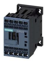
power contactor, AC-3e/AC-3, 16 A, 7.5 kW / 400 V, 1 NC, 24 V DC with integrated diode, 3-pole, frame size S00 spring-loaded terminal
