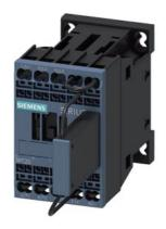
traction contactor, AC-3e/AC-3, 16 A, 7.5 kW / 400 V, 3-pole, 110 V DC, 0.7-1.25\* Us, with integrated suppressor diode, auxiliary contacts: 1 NC, spring-loaded terminal, size: S00, with plugged on series resistor
