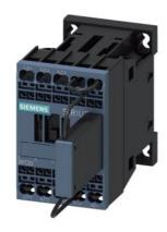
traction contactor, AC-3e/AC-3, 16 A, 7.5 kW / 400 V, 3-pole, 125 V DC, 0.7-1.25  $^{\ast}$  Us, with integrated suppressor diode, auxiliary contacts: 1 NC, spring-loaded terminal, size: S00, with plugged on series resistor
