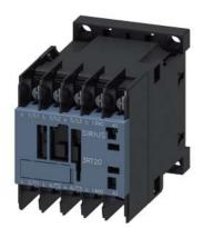
power contactor, AC-3e/AC-3, 7.5 kW/400 V, 1 NO, 110 V AC, 50 Hz, 120 V, 60 Hz, 3-pole, frame size S00, ring cable lug connection
