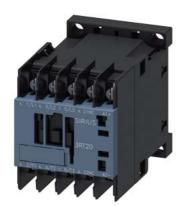
power contactor, AC-3e/AC-3, 16 A, 7.5 kW / 400 V, 3-pole, 24 V DC, auxiliary contacts: 1 NC, ring cable lug connection
