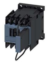
traction contactor, AC-3e/AC-3, 16 A, 7.5 kW / 400 V, 3-pole, 24 V DC, 0.7-1.25  $^{\star}$  Us, with integrated varistor, auxiliary contacts: 1 NC, ring cable lug connection, size: S00, with plugged on series resistor
