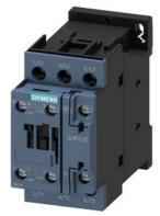
power contactor, AC-3e/AC-3, 9 A, 4 kW / 400 V, 1 NO + 1 NC, 600 V AC, 60 Hz 3-pole, frame size S0 screw terminal
