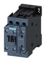
power contactor, AC-3e/AC-3, 9 A, 4 kW / 400 V, 3-pole, 125 V DC, auxiliary contacts: 1 NO + 1 NC, screw terminal
