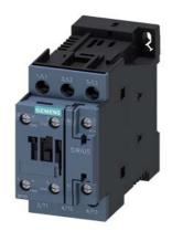
power contactor, AC-3e/AC-3, 9 A, 4 kW / 400 V, 3-pole, 21-28 V AC/DC, 50/60 Hz, with integrated varistor, auxiliary contacts: 1 NO + 1 NC, screw terminal
