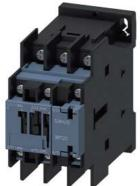
power contactor, AC-3e/AC-3, 9 A, 4 kW / 400 V, 3-pole, 100 V AC, 50 Hz / 100-110 V, 60 Hz, auxiliary contacts: 1 NO + 1 NC, ring cable lug connection, size: S0
