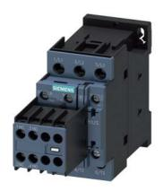
power contactor, AC-3e/AC-3, 12 A,  $5.5\,kW$  / 400 V, 3-pole, 110 V AC, 50 Hz / 120 V, 60 Hz, auxiliary contacts: 2 NO + 2 NC, screw terminal, size: S0, removable auxiliary switch
