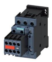
power contactor, AC-3e/AC-3, 12 A, 5.5 kW / 400 V, 3-pole, 110 V AC, 50 Hz / 120 V, 60 Hz, auxiliary contacts: 2 NO + 2 NC, screw terminal, captive auxiliary switch
