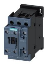
power contactor, AC-3e/AC-3, 12 A, 5.5 kW / 400 V, 3-pole, 400 V AC, 50 Hz / 400-440 V, 60 Hz, auxiliary contacts: 1 NO + 1 NC, screw terminal, size: S0
