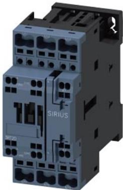
power contactor, AC-3e/AC-3, 12 A, 5.5 kW / 400 V, 1 NO + 1 NC, 110 V AC, 50 Hz 120 V, 60 Hz, 3-pole frame size S0, spring-loaded terminal
