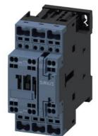
power contactor, AC-3e/AC-3, 12 A, 5.5 kW / 400 V, 3-pole, 400 V AC, 50 Hz, auxiliary contacts: 1 NO + 1 NC, spring-loaded terminal, size: S0
