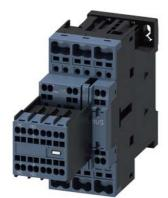
power contactor, AC-3e/AC-3, 12 A, 5.5 kW / 400 V, 3-pole, 400 V AC, 50 Hz, auxiliary contacts: 2 NO + 2 NC, spring-loaded terminal, size: S0, removable auxiliary switch
