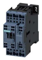
power contactor, AC-3e/AC-3, 12 A, 5.5 kW / 400 V, 1 NO + 1 NC, AC (50-60 Hz) DC operation 21-28 V AC / DC 3-pole, frame size S0 spring-loaded terminal
