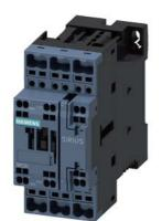
power contactor, AC-3e/AC-3, 12 A, 5.5 kW / 400 V, 1 NO + 1 NC, AC (50-60 Hz) DC operation 95-130 V AC / DC 3-pole, frame size S0 spring-loaded terminal
