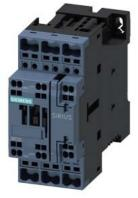
traction contactor, AC-3e/AC-3, 12 A, 5.5 kW / 400 V, 3-pole, 72 V DC, 0.7-1.25\* Us, electronic drive, with integrated varistor, auxiliary contacts: 1 NO + 1 NC, spring-loaded terminal, size: S0
