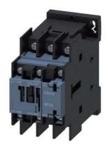
power contactor, AC-3e/AC-3, 12 A, 5.5 kW / 400 V, 3-pole, 400 V AC, 50 Hz / 400-440 V, 60 Hz, auxiliary contacts: 1 NO + 1 NC, ring cable lug connection, size: S0
