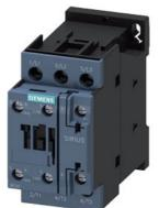
power contactor, AC-3e/AC-3, 17 A, 7.5 kW / 400 V, 1 NO + 1 NC, 230 V AC, 50 / 60 Hz, 3-pole, screw terminal
