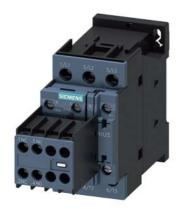
power contactor, AC-3e/AC-3, 17 A, 7.5 kW / 400 V, 3-pole, 400 V AC, 50 Hz, auxiliary contacts: 2 NO + 2 NC, screw terminal, size: S0, removable auxiliary switch
