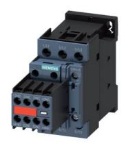
power contactor, AC-3e/AC-3, 17 A, 7.5 kW / 400 V, 3-pole, 110 V AC, 50 Hz / 120 V, 60 Hz, with plugged-in varistor, auxiliary contacts: 2 NO + 2 NC, screw terminal, size: S0, captive auxiliary switch
