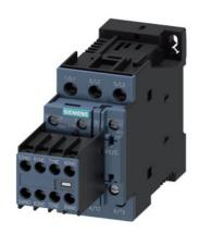
power contactor, AC-3e/AC-3, 17 A, 7.5 kW / 400 V, 3-pole, 24 V DC, with plugged-in diode combination, auxiliary contacts: 3 NO + 3 NC, screw terminal, with 3RH2911-1XA22-0MA0
