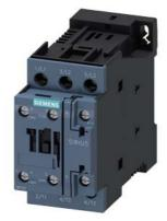
power contactor, AC-3 17 A, 7.5 kW / 400 V 1 NO + 1 NC, AC (50-60 Hz) DC operation 95-130 V AC/DC, 3-pole, Size S0, screw terminal
